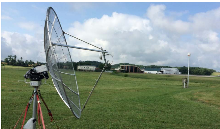
Figure 1. A high gain parabolic dish system for tracking GNSS satellites.
