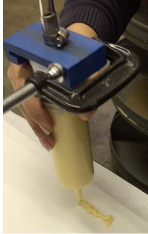
Figure 2. Preliminary conceptual design for extrusion testing.
