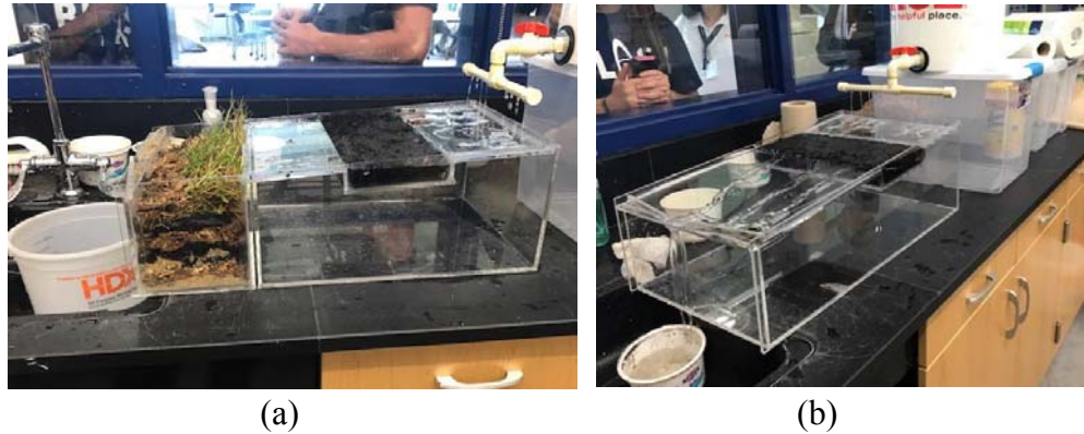
Figure 4. (a) Unit with mixed-media bioretention system; (b) Unit without bioretention system.
