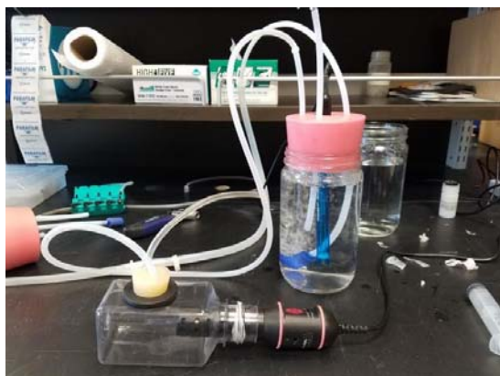
Figure 6. Experimental setup for acidification session, including a pH probe inserted through a stopper into a glass jar into which CO 2 was allowed to flow, and a CO 2 sensor, which measured CO 2 concentration in air that was displaced from the glass jar.
