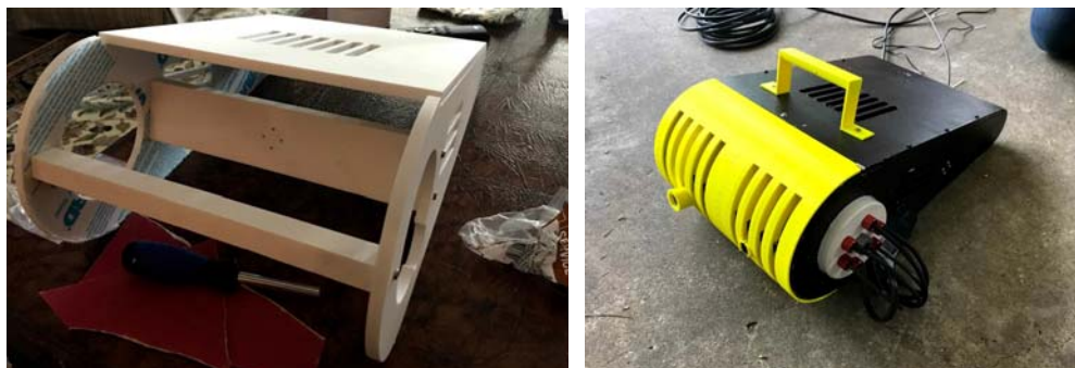
Figure 10: ROV housing and PVC cap with cable penetrators and completed ROV
