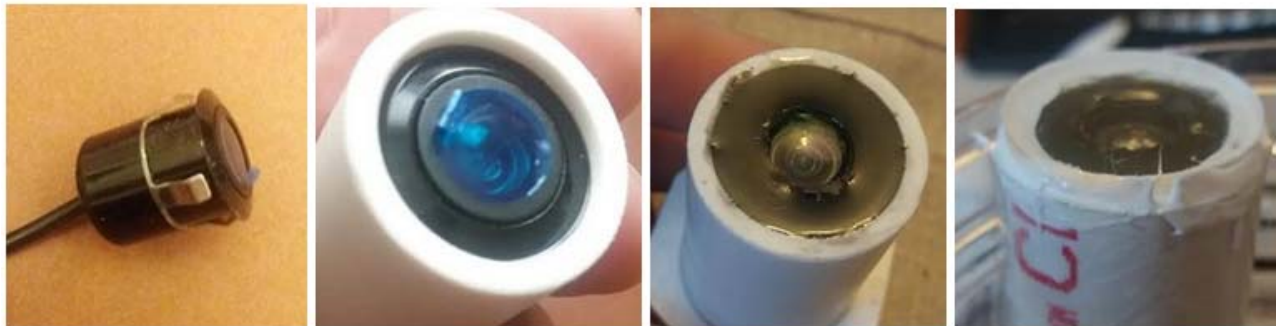
Figure 4: Parts of the camera assembly left to right: Camera, camera in pvc housing, potting material applied, acrylic lense in place with JB weld
