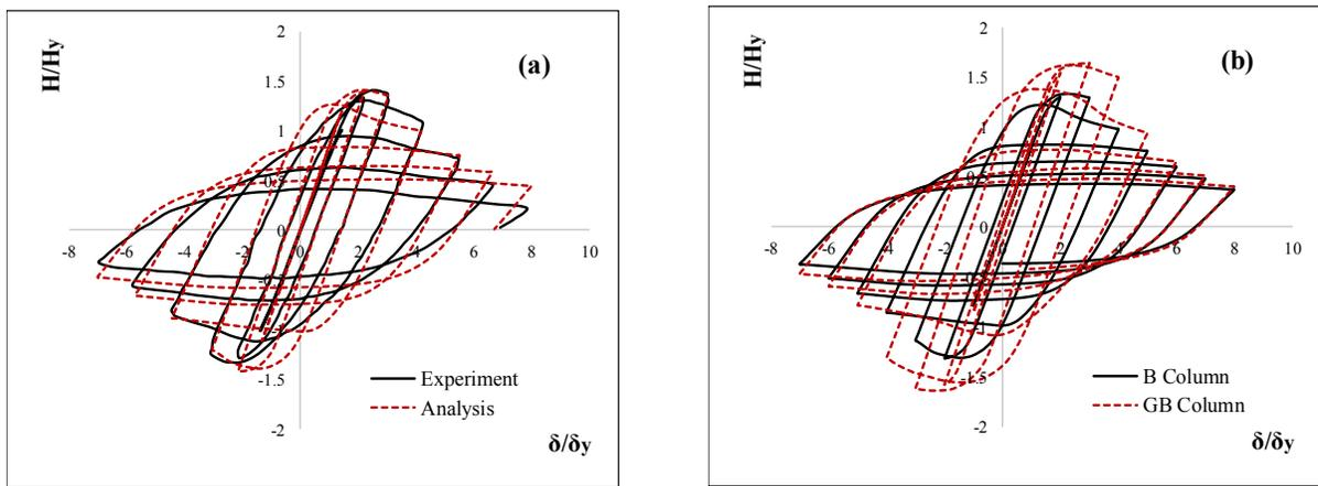
Figure 3. Comparison of lateral load vs. lateral displacement hysteresis curves.
