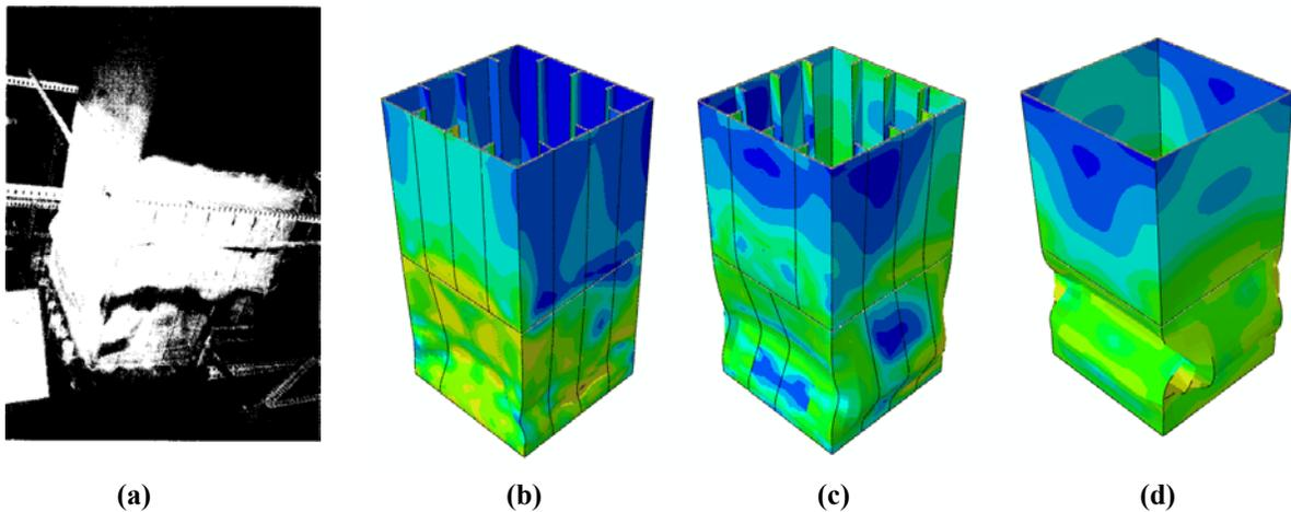
Figure 4. Buckling shapes of columns: (a) experiment\*, (b) B column with stiffeners, (c) GB column, and (d) B column without stiffeners. (\*reported in Nishikawa et al., 1998)
