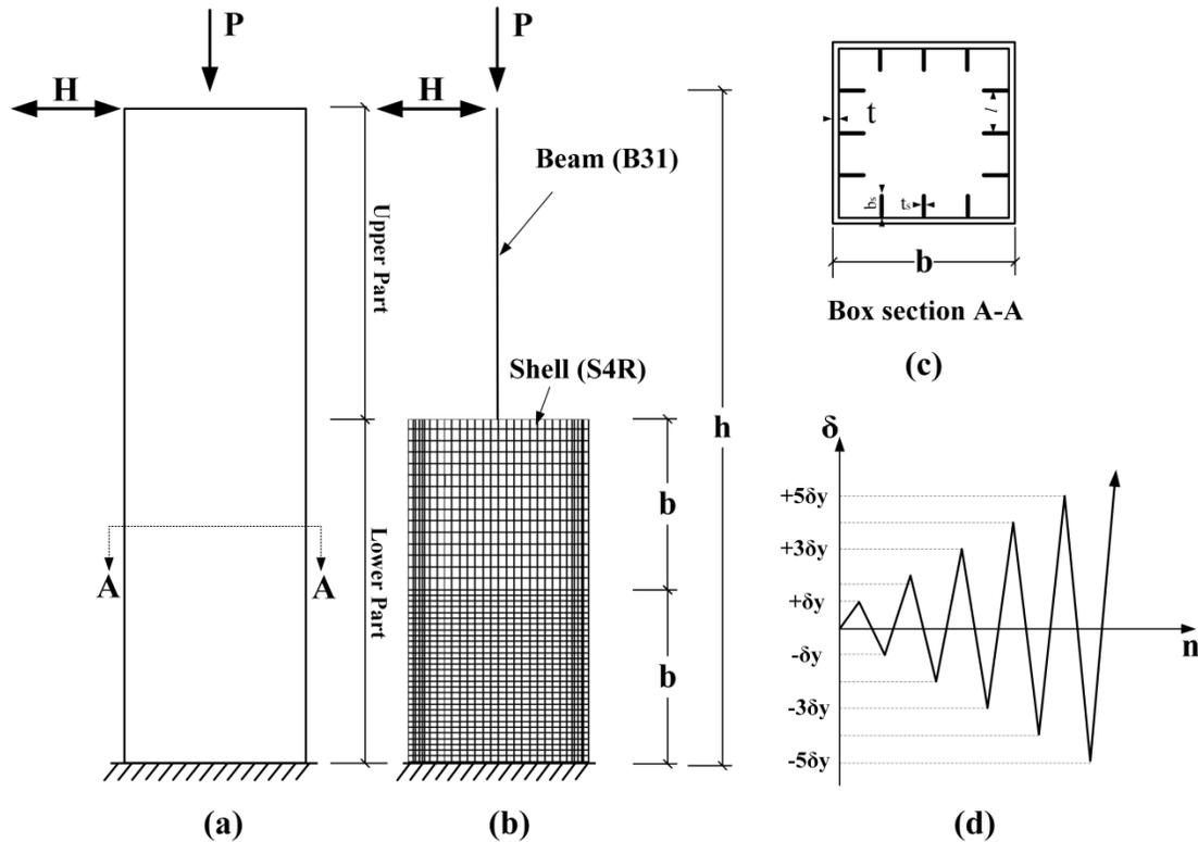
Figure 1. B Column model: (a) column; (b) FE meshing; (c) cross section; and (d) loading program.
