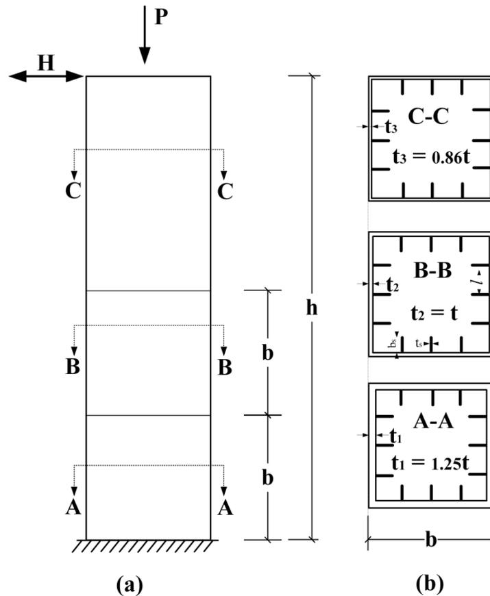
Figure 2. GB Column model: (a) column, and (b) graded-thickness sections.
