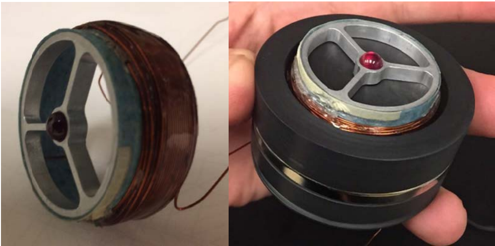
Figure 8. Voice Coil and Operator (left) Inserted into Outer Shell Assembly (right)
