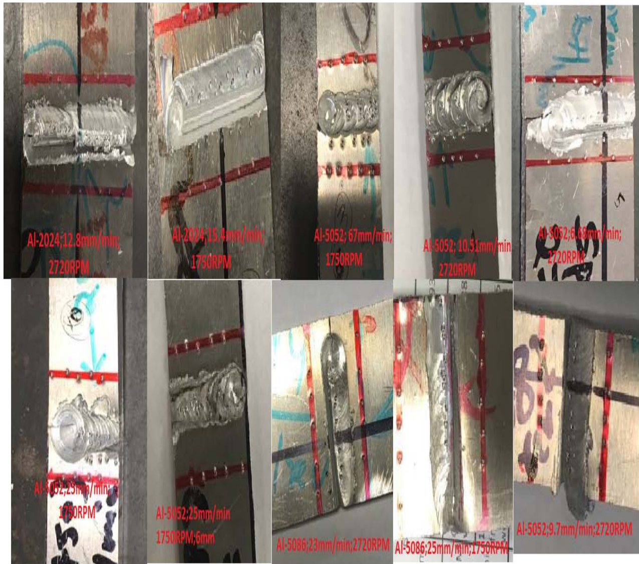
Figure 12. All experimented work piece pictures with their material name, feed rate, and tool speed.
