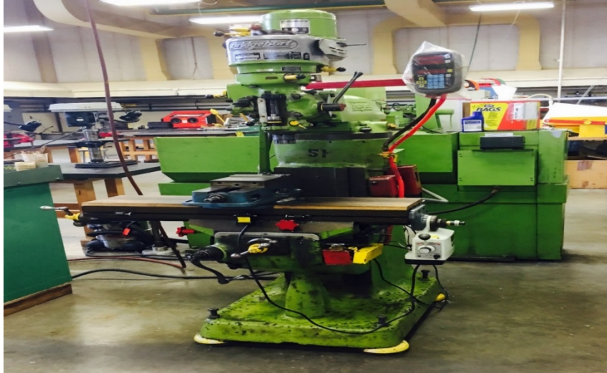
Figure 6. 1½ HP J head Bridgeport-vertical milling machine.
