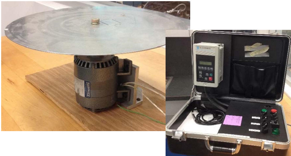
Figure 1. Photographs of original turntable and portable VFD.
